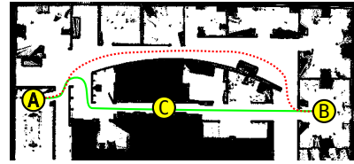
Fig. 7. Experimental setup for the path planning experiment. The task consists in navigating between A and B . At C we added a virtual door that changed its state over time.
